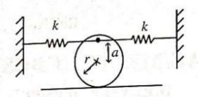
a) Determine the natural frequency of the system shown in figure by energy and Newton's method.
